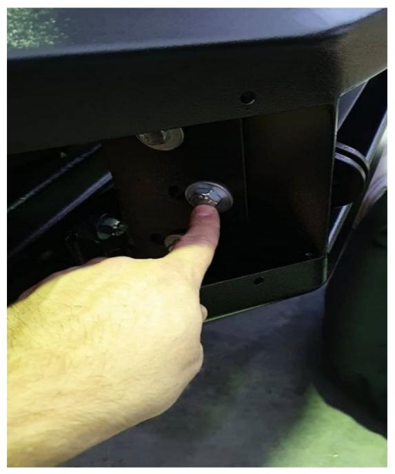
5) The black inner guards need to be trimmed to suit the profile of the bulbar and be secured in place so they do not move around.
