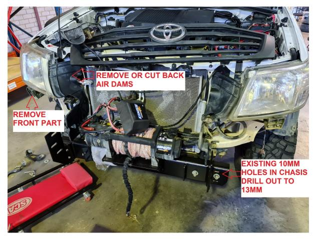
2) Install the cradle onto the chassis rail ends. Bolts should be finger Tight as you need to align the bulbar later.
