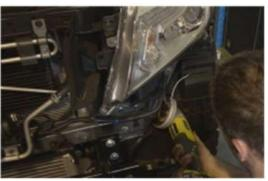
8. Carefully mount the Extreme Series bar it is best to get someone to help you. The bulbar alignment can be difficult. Its best to have bolts loose enough so two persons can hold the bar in place while a 3<sup>rd</sup> tightens the bar. If you are installing by your self alignment can be difficult its suggested you tighten 1 side enough so it can still move under pressure and wedge foam (or similar) between bar and fender to retain gap when lifting the other side
