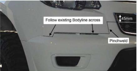
3. It is suggested you remove the front grille off the car inorder to make the final cut shown below. You will need to remove the 2 barbs either side under the head lights with bolt cutters
