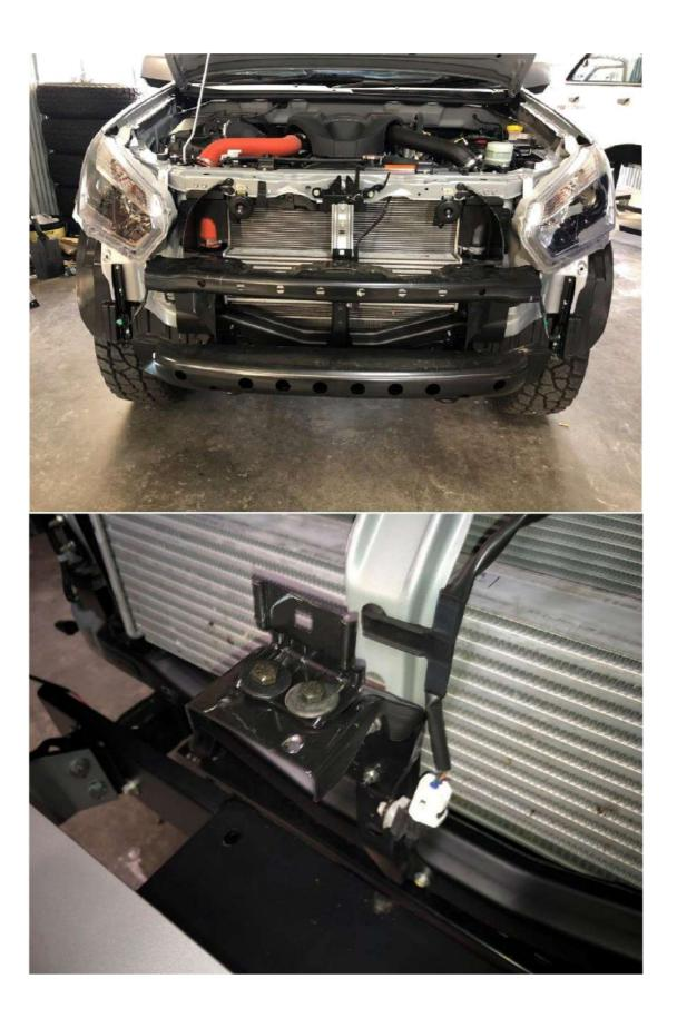
If you need further adjustment left to right you may need to flatten the bump on the chassis front member & install the Chassis collar bracket.
