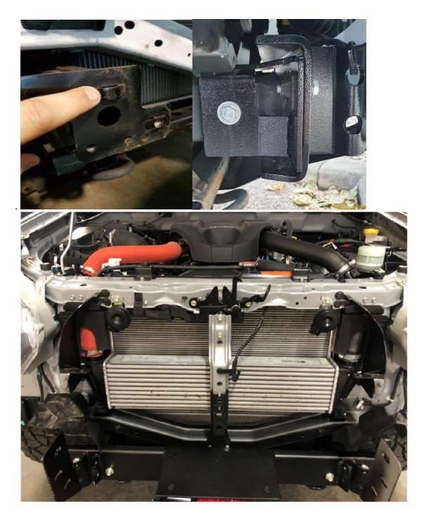
We recommend the use of 10mm foam on the sides between the bar and the car to help get the bar even.
