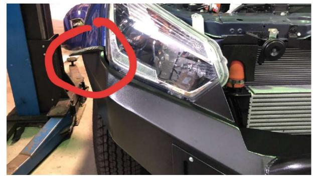
Typically, we cut the grille and apply some flat style pinch weld to get the bar nice and close to the car
