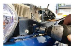
6. Undo the bolts hoding the inner wheel liner to the bumper.
