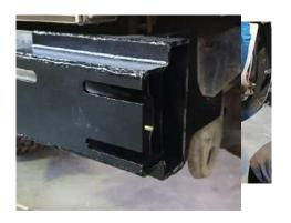
12. Now mount the winch cradle to the bolts in the adaptor brackets. You will need a long spanner to hold the bolt head while you tighten the lock nuts from the front.
