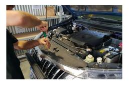
3. With the grill cover removed, you can remove the two screws holding the top of the grill to the radiator support.
