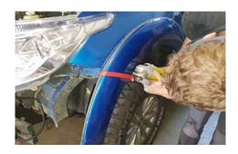
20. With a helper, mount the bar to the bracket, taking your time to ensure the bar is level.
