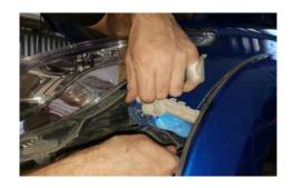
14. Remove the factory washer bottle located under the passenger side headlights. You will be left with the wiring and the water hose loose as seen in the photo.
