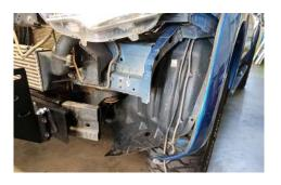
15. Mount the new washer bottle bracket as shown. The bracket fits between the bonnet stop and the bonnet stay clip.
