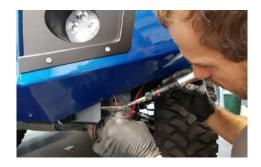
23. With the bar mounted, ensure that there isn't any stress on the washer bottle hose or wiring and tidy with cable ties.
