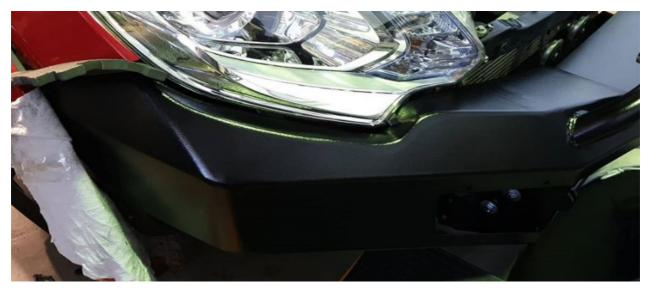
This will create an even gap on both sides, vs trying to align 1 side at a time. We also recommend using same foam under the head lights to maintain the correct gap
