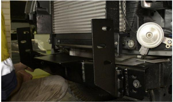
3) We recommend you bolt on cradle finger tight enough so you can move the cradle left to right if you need too. Use 10-15mm foam (clark rubber) or cardboard of equal depth and tape to the bulbar where bar meets guards, use a tape which does not affect the paint. See images below typical image
