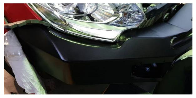
This will create an even gap on both sides, vs trying to align 1 side at a time. We also recommend using same foam under the head lights to maintain the correct gap
