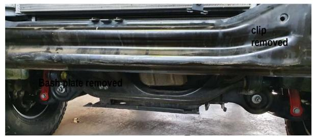
Now install the cradle centred with the 2 outer bolts on each side, you can use the 3 plastic tabs on the car infront of the radiator as centre link. The cradle is approx. 1100mm long & centre point is approx. 550mm
