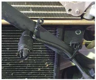
3) If you have metal bash plate simple drill through and mount bolts on the angle, ensure you mount bolt close as far in as possible.
