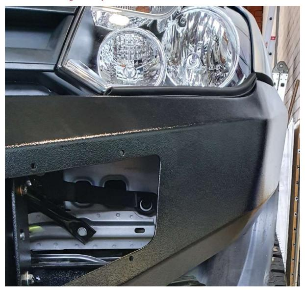
10) Install centre bolts through fog light opening first which allow you to line up bulbar better. Once aligned in place now install remaining bolts.
