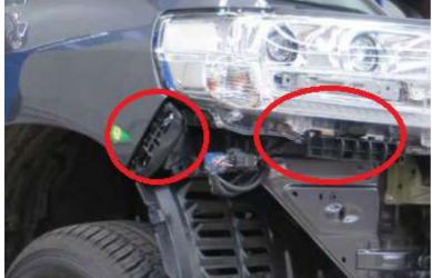
4) Fit mounting hardware, The spacer brackets first then the cradle. The spacer brackets can be tight but keep cradle loose incase you need to move left or right
