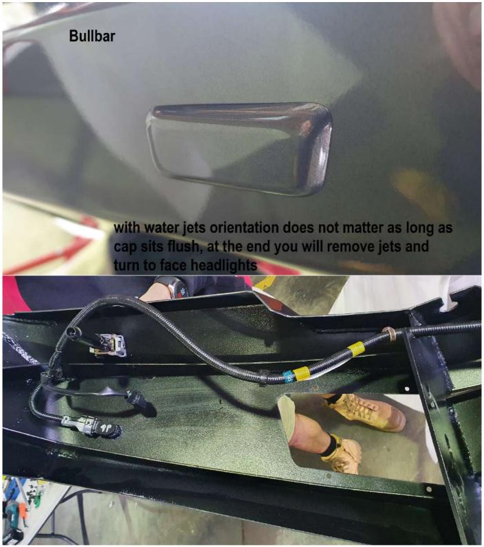
7) Put the harness in place, You will cable tie the harness to the rib supports in the bulbar, small slots should exist in various points of the bulbar to slide a cable tie in, otherwise you can purchase adhesive retainers (not supplied) Just ensure your supplied LED fog lights have enough cable to reach the existing harness, the new LED spot lights may require you to connect upside down, EG flip connector upside down and plug into harness if LED not working.
