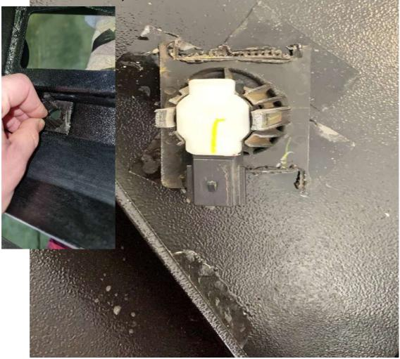
7) Finally make sure you secure the grille back into place so it can not flap around by cable tying the grille to nearest support firmly. Depending on what
