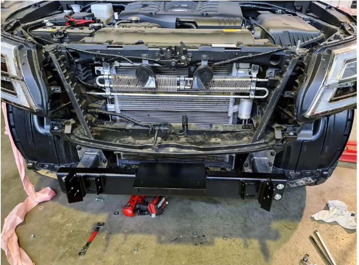
Remove the air dams near head lights or you can trim to suit profile of the bar which only possible by putting bar on marking and removing. If you are fitting a winch unbolt the middle support bracket in the centre of the car above winch plate – Fits runva 11xp premium height.
