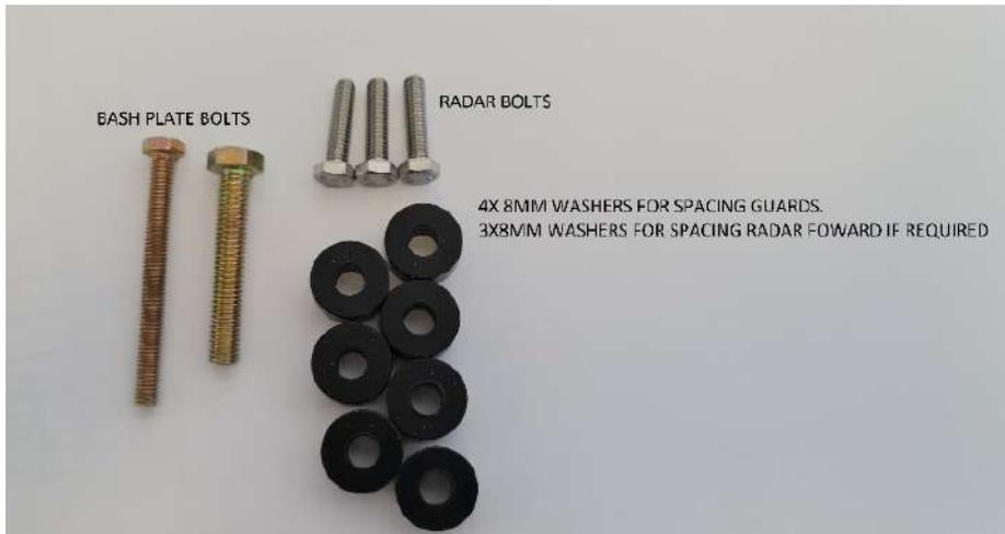
spacing guards to suit bar - each side of guard is held in with 2 bolts, remove bolts and install washer x2 each side as per below. use the longer factory bolts you removed from bumper in lieu of original bolts as they are too short.
