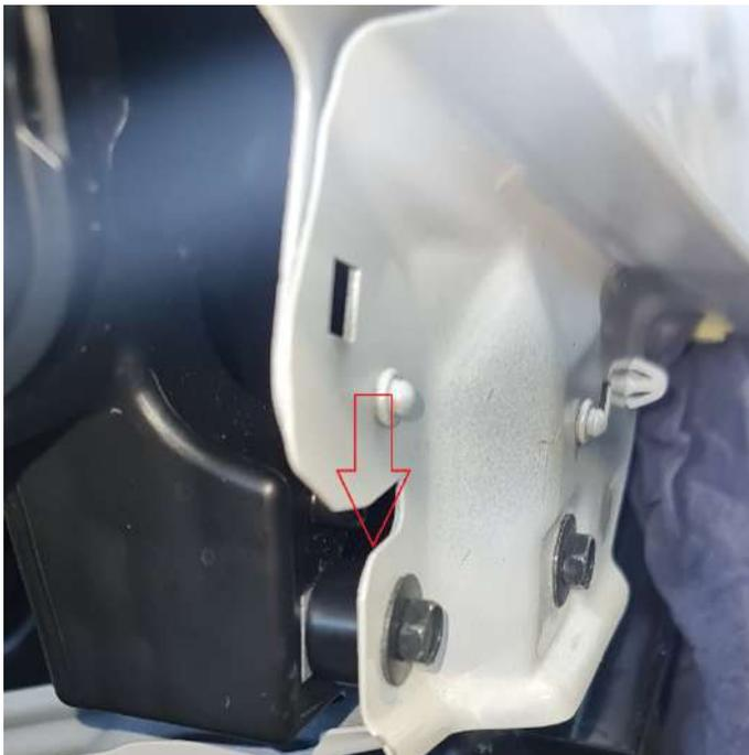
Bash Plate : you will need to install a rivnut on drivers side to secure bash plate.
